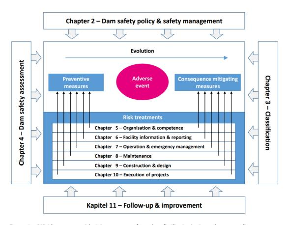
Figure 1. RIDAS structure with risk treatments for a dam facility in the inner box, as well as general conditions, classification, dam safety assessment and follow-up.
