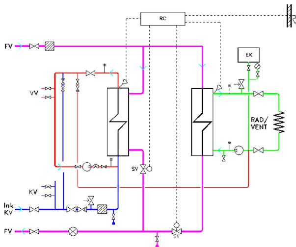
Parallel connection is an arrangement of district heating substation connections in which the heat exchangers are connected in parallel across the supply's incoming and return connections. One heat exchanger supplies the radiator circuit, and the other supplies the domestic hot water circuit. This arrangement is that which is most commonly used.
