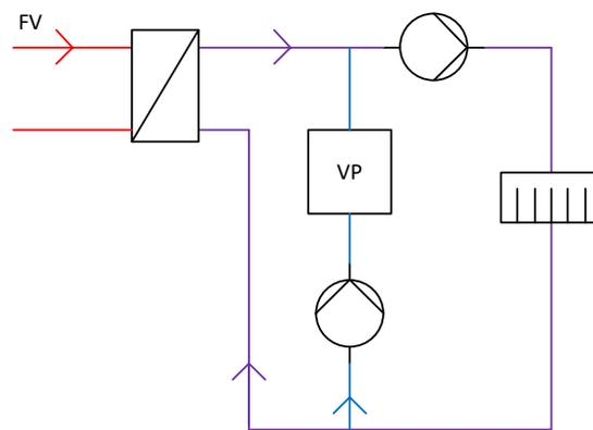
**In this arrangement, the heat pump supplies only space heating. It and the district heating supply are connected in parallel.**
