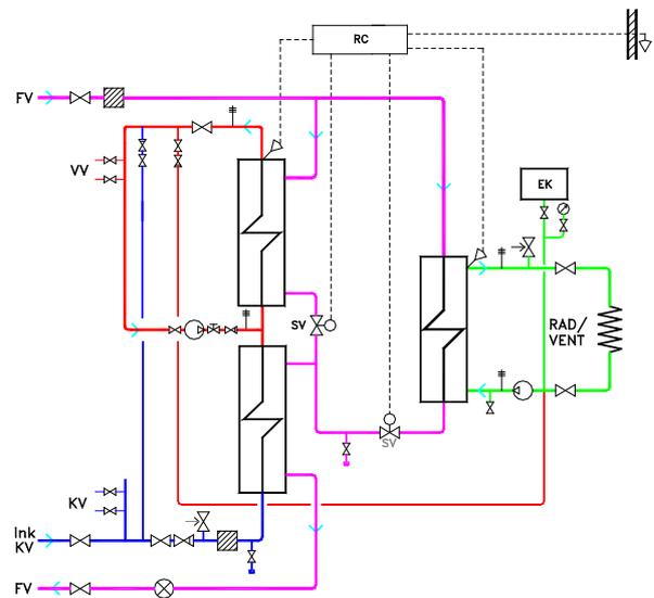
Two stage connection is also commonly used. The return water from the radiator circuit heat exchanger is used to preheat the domestic hot water. The proportions of heat supplied as pre-heating and post-heating respectively are set in such a way as to make best use of the return temperature from the radiator circuit. If the building has a substantial demand for hot water, this connection arrangement generally results in a lower return temperature than from parallel connection.
