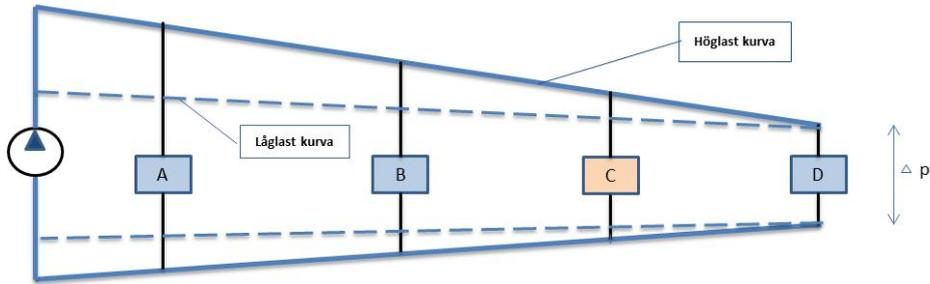
**Figure 2.** An example of the ranges over which the differential pressure in a district heating system can vary. The distance in the x-plane represents the distance from the system circulation pumps.
