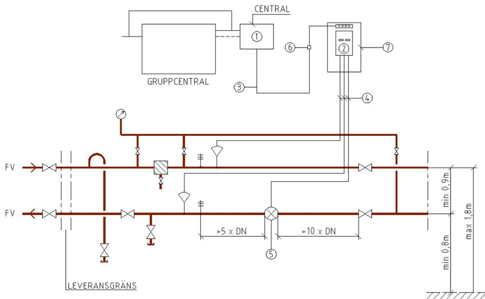
**Figure 5. Schematic diagram of the meter position.**
