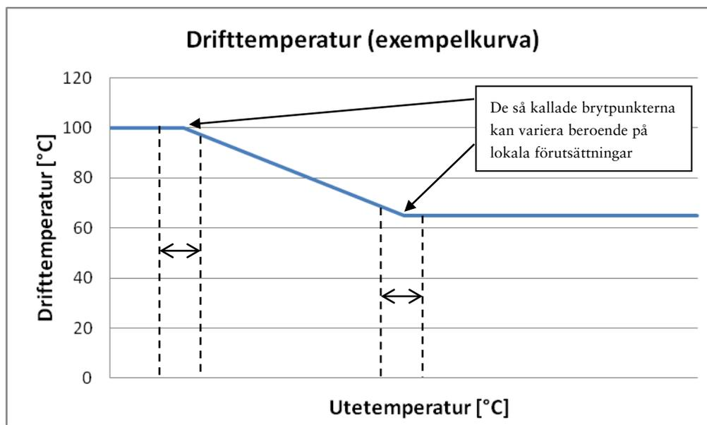
Figure 1. An example of a temperature curve showing the district heating system's operating temperature as a function of the ambient temperature.
