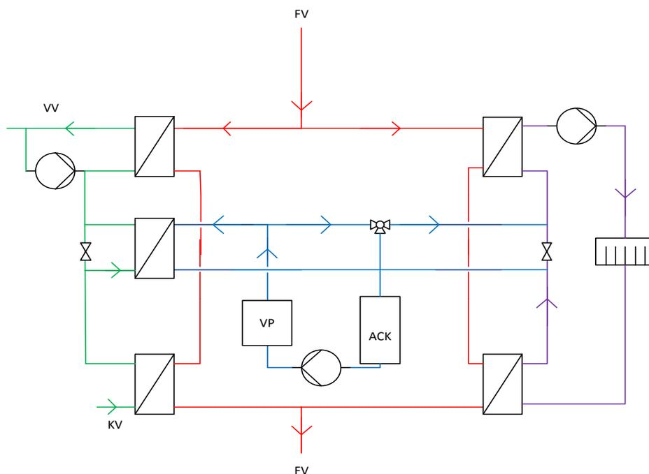
Space heating and domestic hot water in parallel, both produced in three stages with district heating providing pre- and post-heating, with a heat pump as an intermediate stage.
