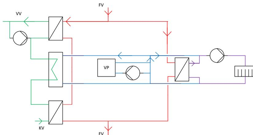
Domestic hot water produced in three stages, with district heating as the preheating and post-heating stages, and the heat pump as an intermediate stage. Space heating is provided by the heat pump and district heating in parallel.
